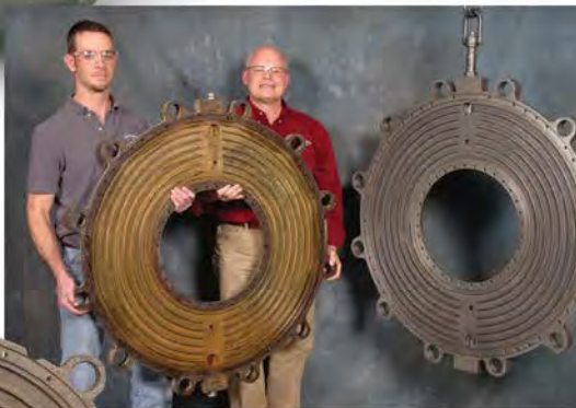
A new 36" composite water jacket (above, left) weighs approx. 95 lbs. A comparable 36" cast iron jacket (above, right) weighs approx. 375 lbs.
